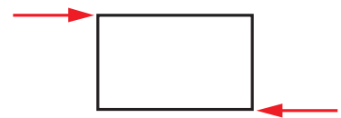
Figure 4.26 The turning effect of two forces acting on a block
