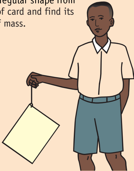
Figure 4.31 Finding the centre of mass of a planar object
